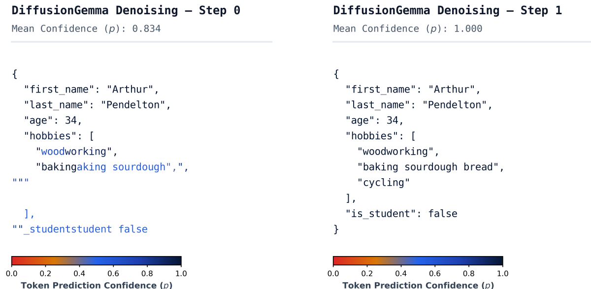
Figure 27 | DiffusionGemma structured generation. Per-token prediction confidence across denoising steps for a JSON output task. Color encodes model confidence p . Because the target output is heavily dictated by the provided JSON schema, text diffusion leverages parallel generation to converge almost instantaneously. The initial canvas (left) is largely correct and exhibits an average confidence exceeding 83% per token. By the second denoising step (right), the output has fully converged to 100% confidence, allowing the final response to be returned in just two steps.
