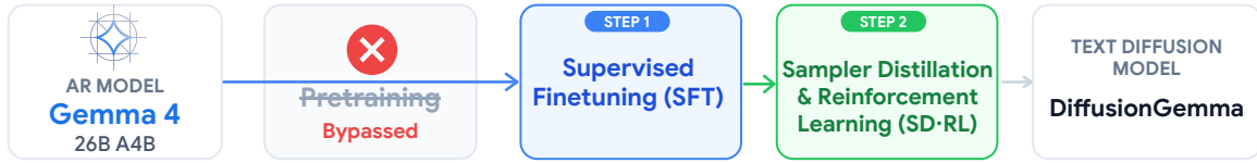
Figure 2 | Overview of our two-stage training pipeline that converts an autoregressive model (Gemma 4 26B A4B) into a text diffusion model (DiffusionGemma). Initialized from the AR model weights, the model first undergoes SFT that adapts it to discrete text diffusion and bidirectional attention across 256-token canvases. This is followed by an online sampler distillation and reinforcement learning phase, which jointly maximizes reward-driven generation quality and compresses the denoising steps to unlock ultra-low latency.
