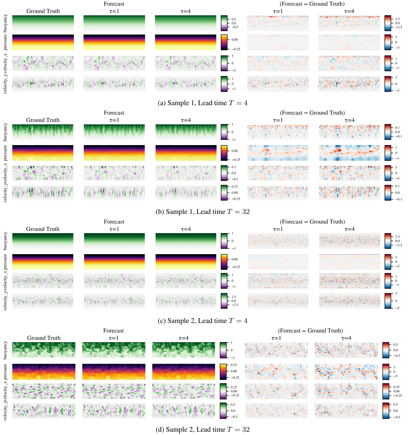
Figure 14: Qualitative examples comparing different time strides on two validation samples from the Rayleigh-Bénard dataset. For models trained with a stride \tau = 4 , visibly increased errors are observed as early as lead time T = 4 and persist at T = 32 .
